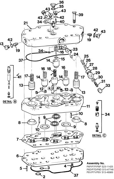
FIGURE 10 VALVE BLOCK ASSEMBLY (Before 7-93)
