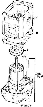
See figure 6: Install the three face plate pins (1) in the holes provided in the barrel face.
