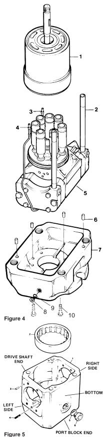
See figure 4: Insert tube line assemblies (3 and 4) in the holes provided in cradle. Note: Tube assemblies must be a snug fit into holes in cradle. Expand end of tubes with a pointed tool to assure fit.
