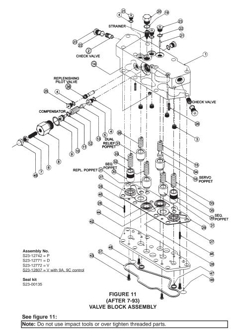
Wash and dry all parts. During assembly, lapped and ground surfaces should be kept lubricated with clean oil and protected from nicks or surface damage.
